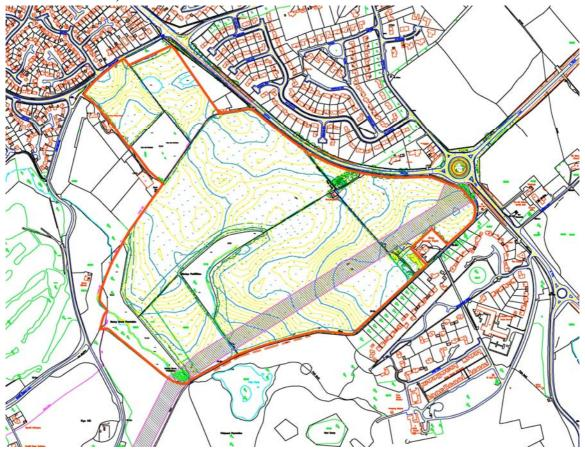
For most developments (under 5 hectares) GPS is not necessary and we would not advise the additional expense. However, there may be a requirement to relate the survey to Ordnance Survey grid and datum by GPS especially if there is a risk of flooding, regardless of the size of the development.
